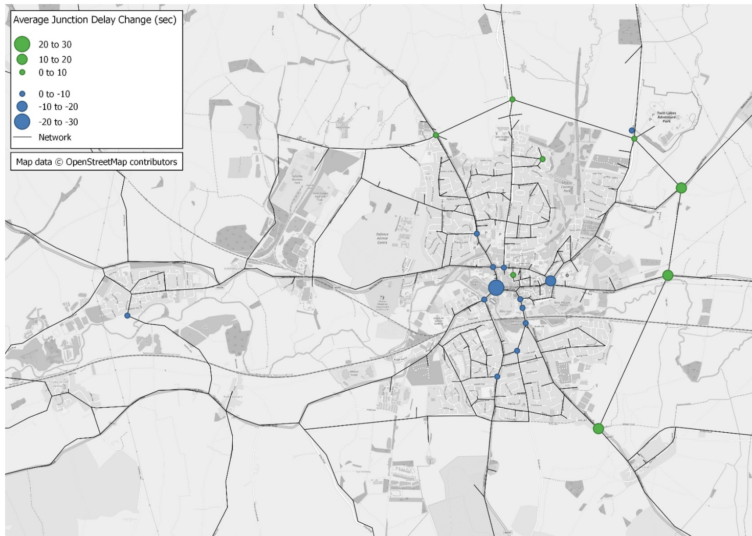
Figure G-3: Forecast Change in Average Delay at Junctions from Core Scenario to NEMMDR Scenario – 2025 PM Peak
