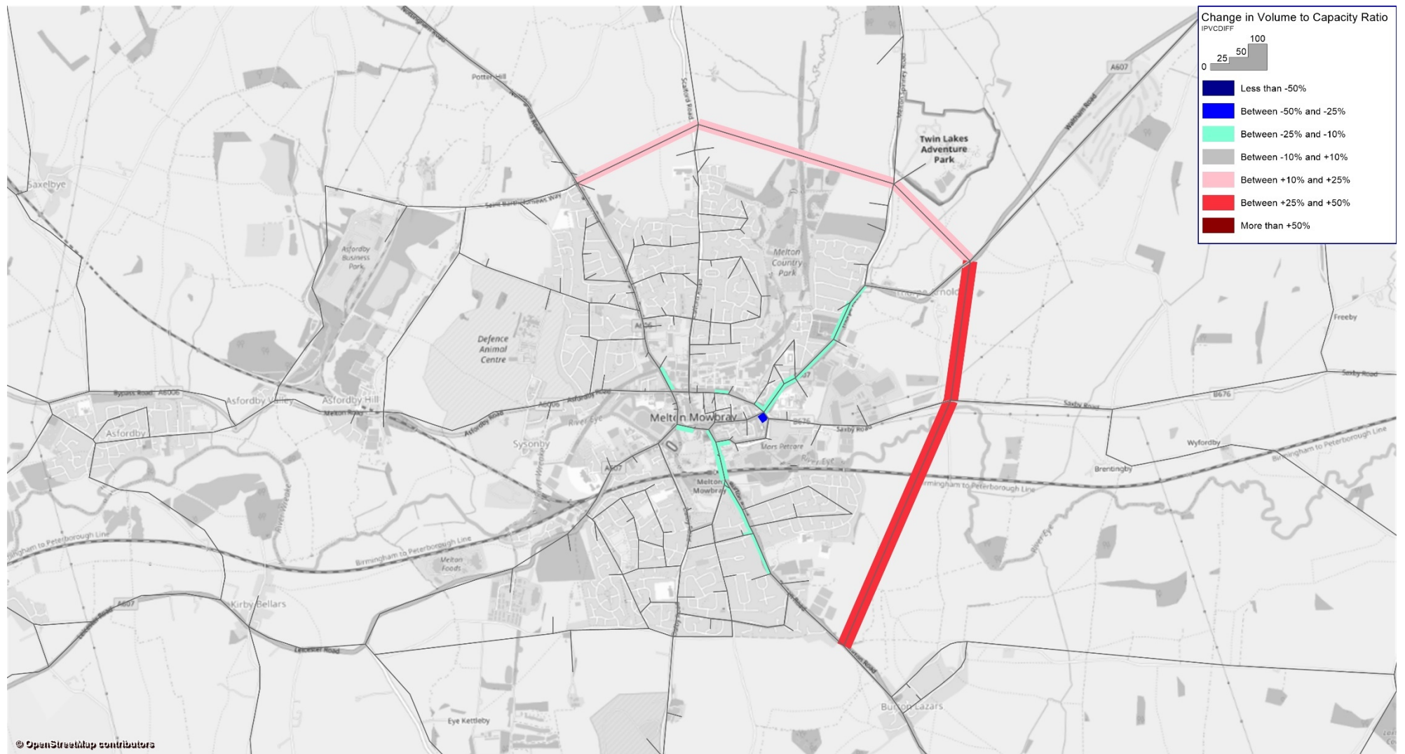
Figure F-2: Forecast Highway Volume-Capacity Ratio Changes from Core Scenario to NEMMDR Scenario – 2025 Interpeak
