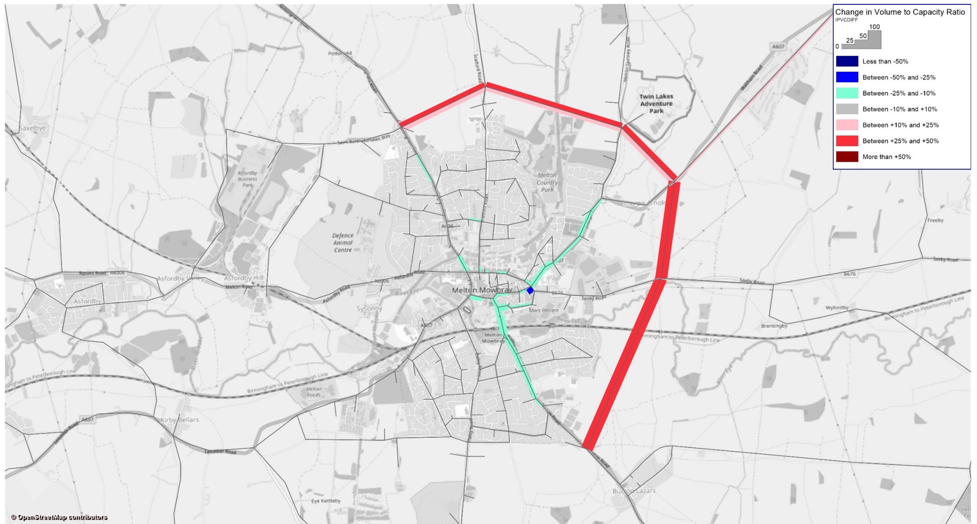
Figure F-5: Forecast Highway Volume-Capacity Ratio Changes from Core Scenario to NEMMDR Scenario – 2030 Interpeak
