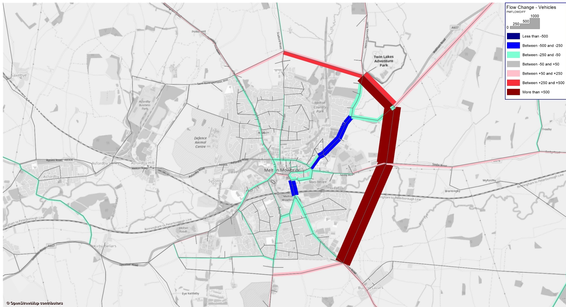
Figure 5-4: Forecast Highway Vehicle Flow Changes from Core Scenario to NEMMDR Scenario – 2040 PM Peak
