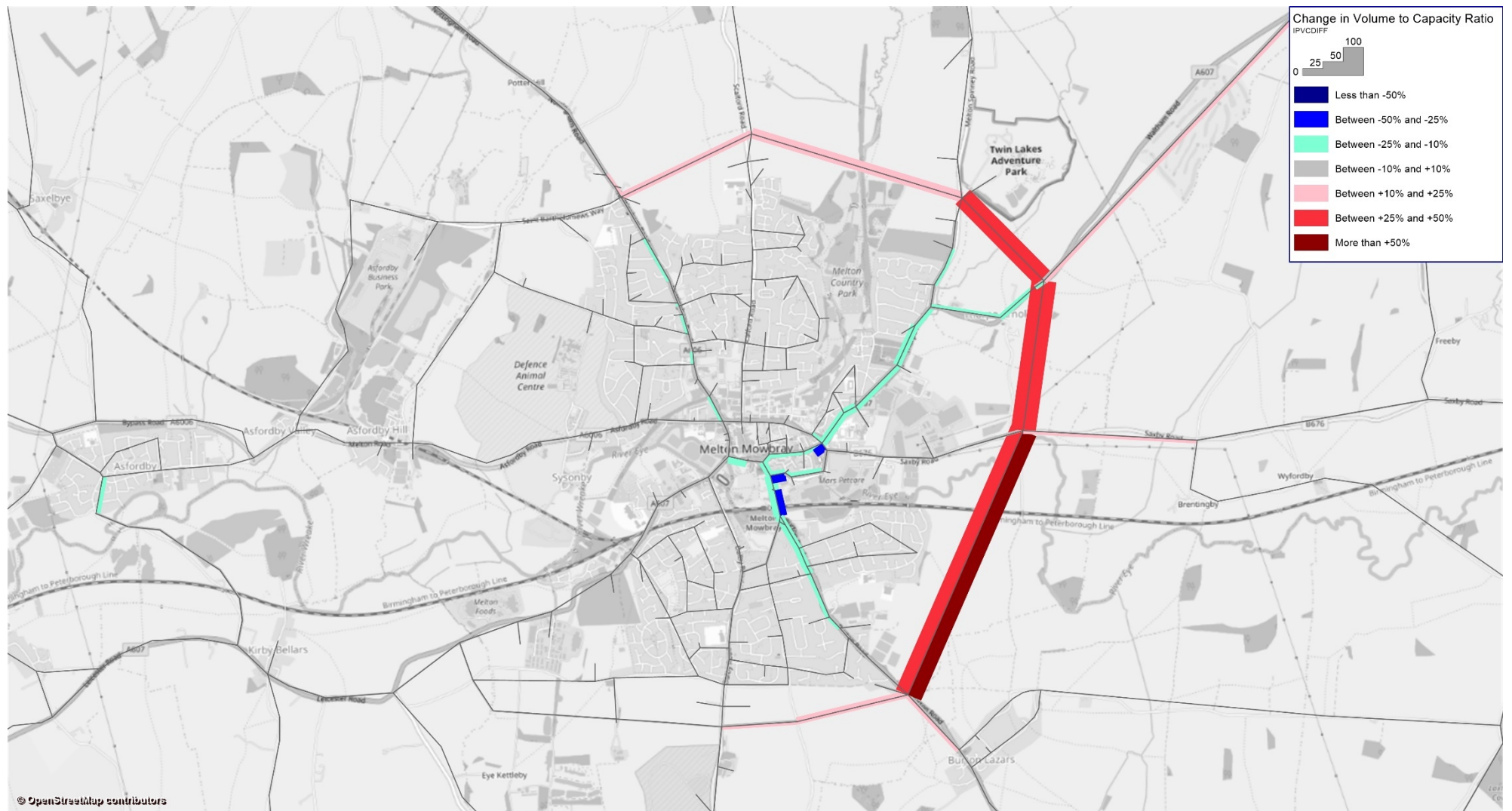
Figure F-11: Forecast Highway Volume-Capacity Ratio Changes from Core Scenario to NEMMDR Scenario – 2051 Interpeak
