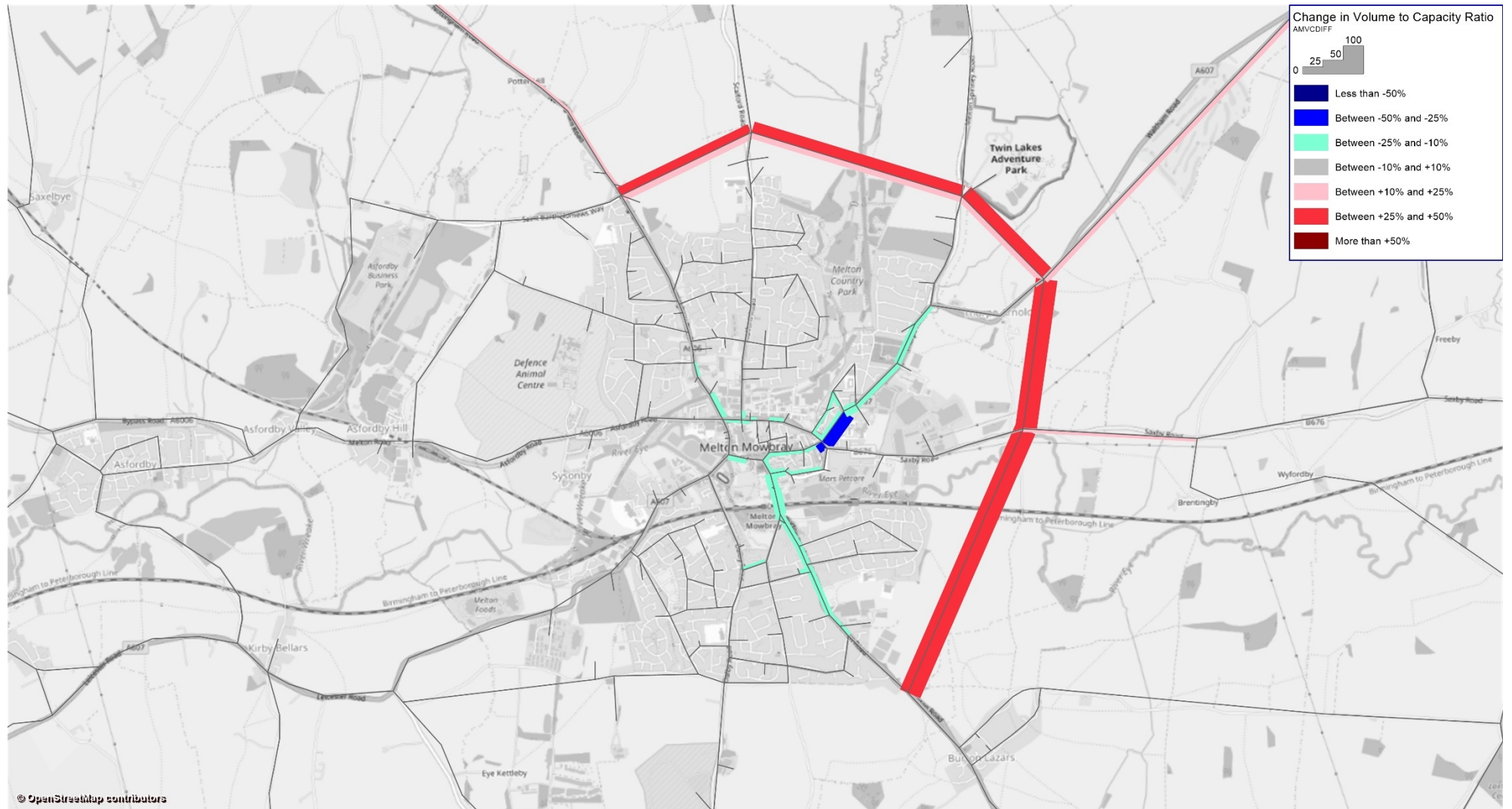
Figure F-1: Forecast Highway Volume-Capacity Ratio Changes from Core Scenario to NEMMDR Scenario – 2025 AM Peak
