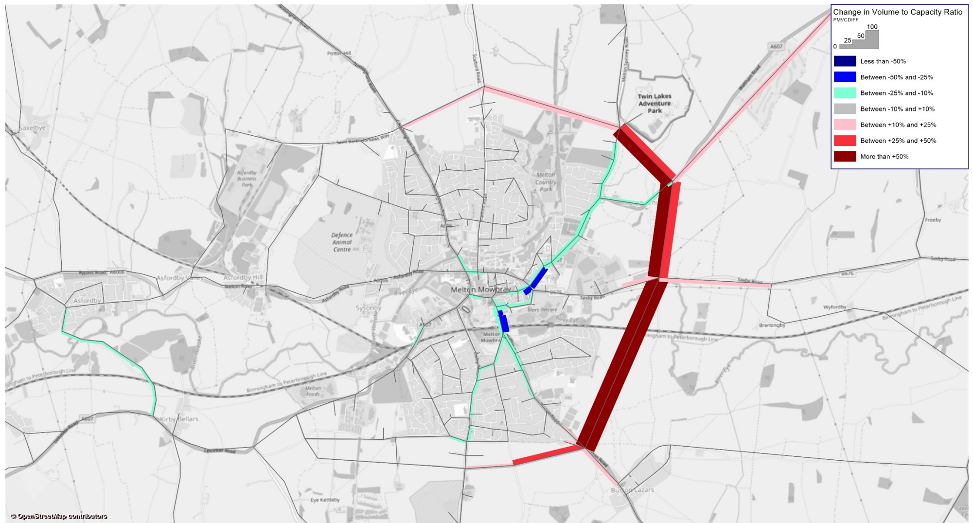
Figure 5-6: Forecast Highway Volume-Capacity Ratio Changes from Core Scenario to NEMMDR Scenario – 2040 PM Peak
