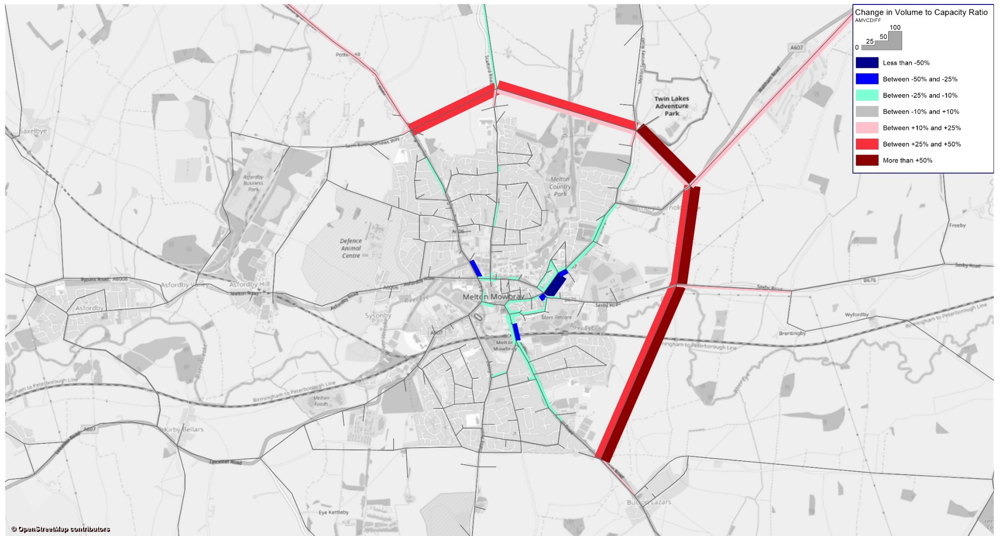
Figure F-4: Forecast Highway Volume-Capacity Ratio Changes from Core Scenario to NEMMDR Scenario – 2030 AM Peak
