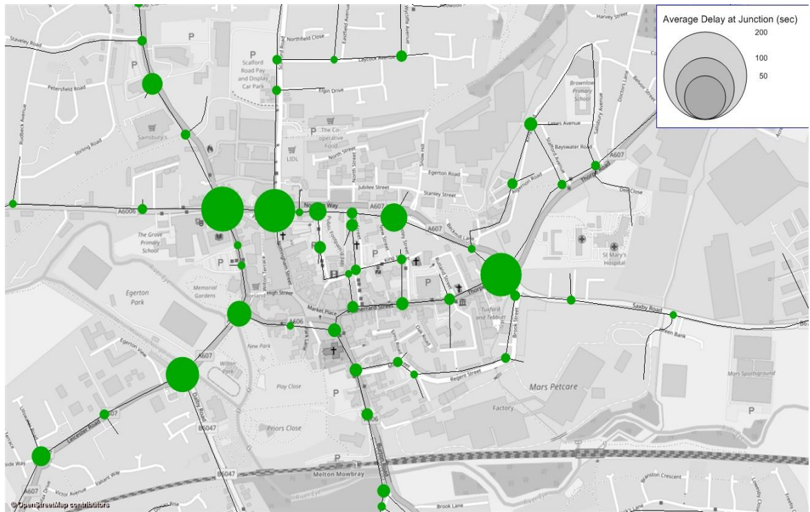
Figure 2-4 Node delays in the AM Peak in Melton Mowbray Town Centre in 2014
